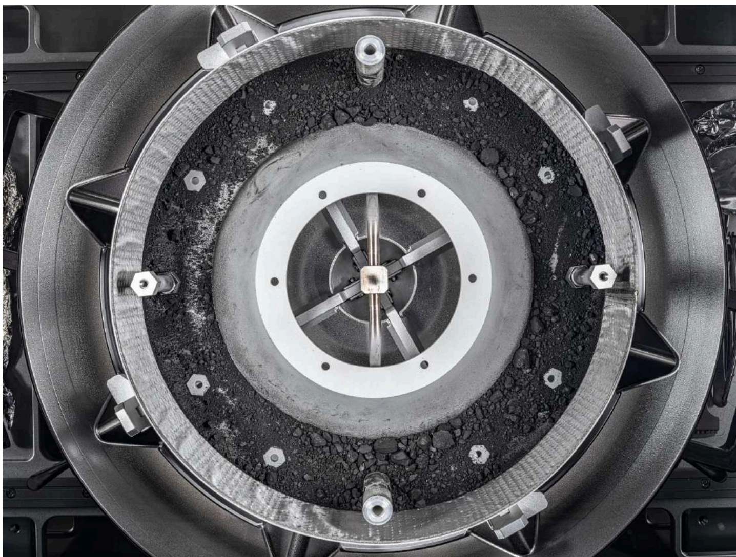
Image of the Touch-and-Go-Sample-Acquisition-Mechanism (TAGSAM) of OSIRIS-REx that collected the asteroid sample on Bennu. Credit - NASA / Erika Blumenfeld & Joseph Aebbersold
